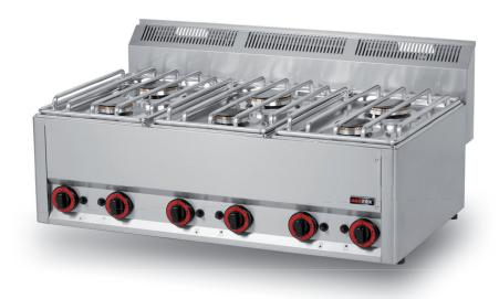
Upper plate thickness 0,8 mm from AISI 304, the rest AISI 430 • High resistance quality burners with performance • Stainless grid from AISI 304 with 10 mm diameter poles • Control only with the regulation knob. • Safety element – thermocouple • Pressed top plate enables comfortable maintenance • Fan assisted oven GN 1/1, inserts with 5 guiding bars • Temperature regulation 50-300 °C, safety thermostat 360°C • In module 990 mm timer 90 min • Stainless chimney
